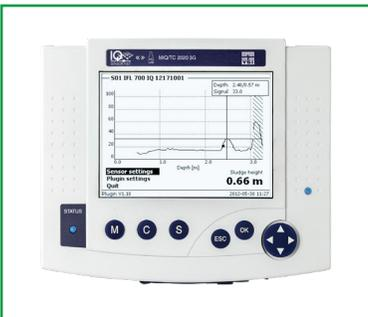
A graphical display of the sludge profile allows operators to visualize sludge height, providing a better understanding of the process and optimized control.
